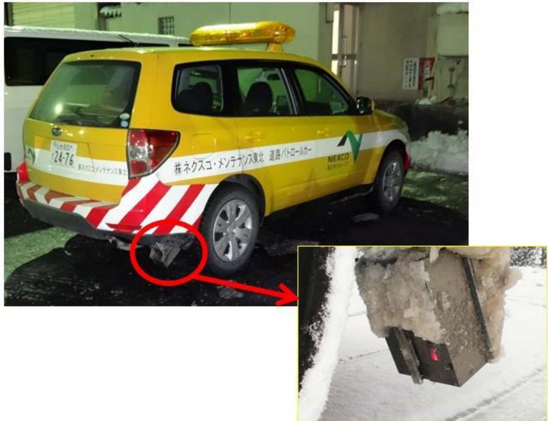
Vehicle fitted with salinity sensor in Japan
