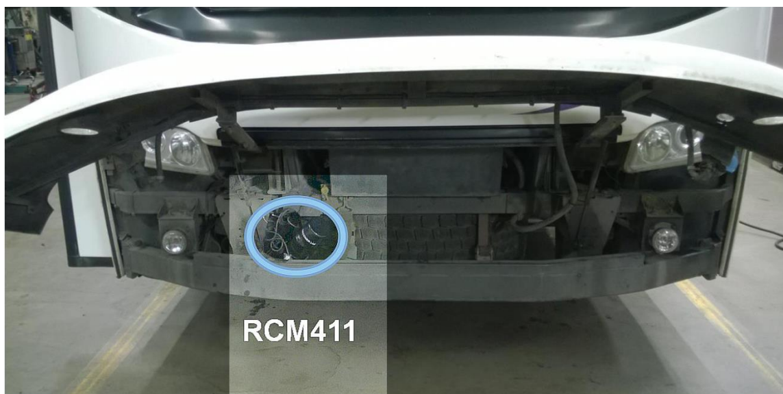
Mobile road condition monitor installed in a bus
