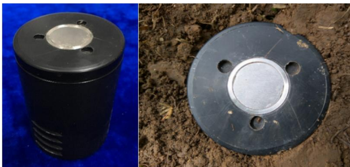
The picture of the wireless ice sensor buried underground
