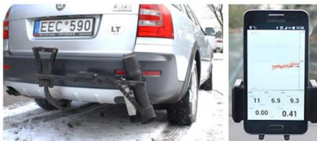
Mobil optical friction measurement device used by a technical road supervisor
