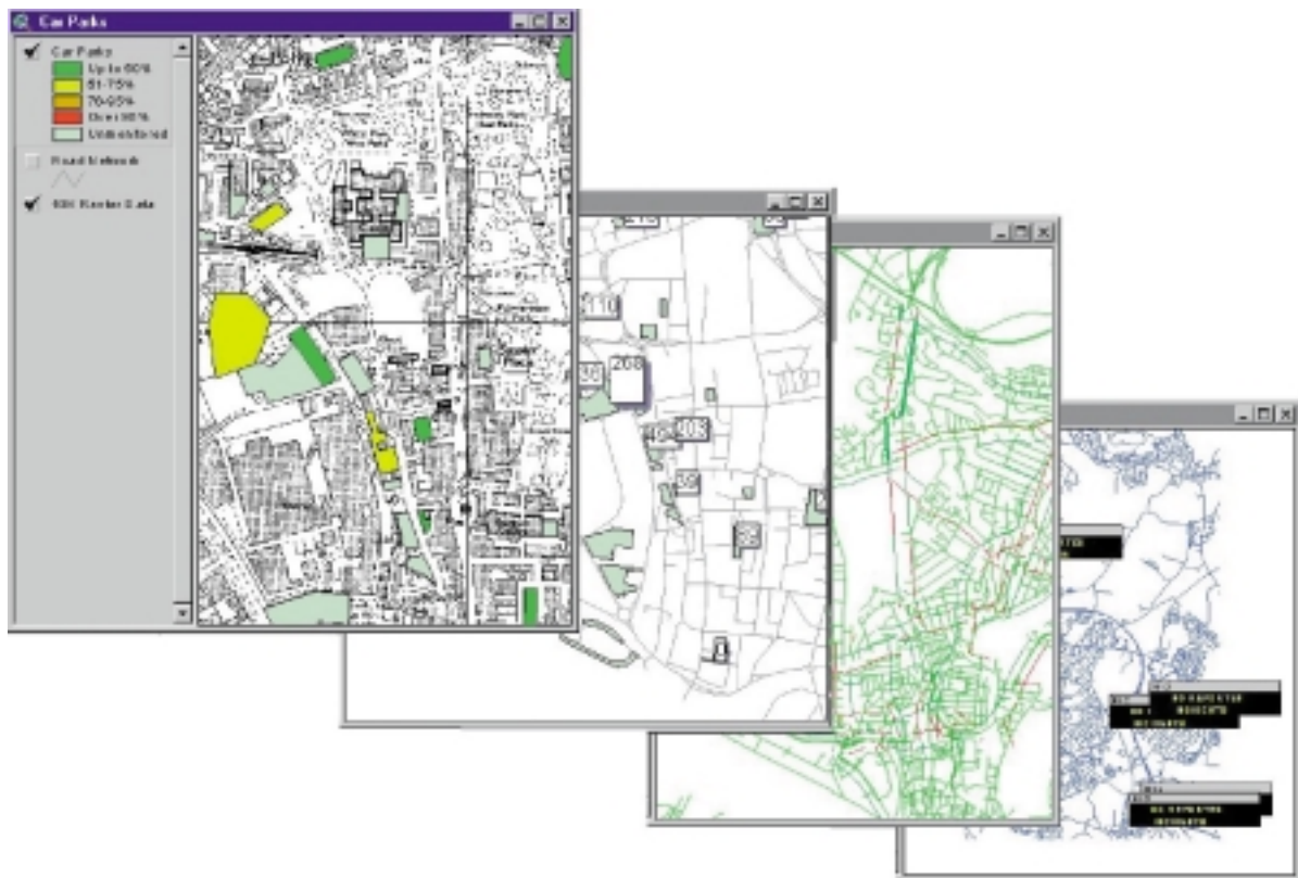
Example of various GIS Layers at different scales. Based on Ordnance Survey mapping ©Crown Copyright. All rights reserved. MEDIA/251/00.
